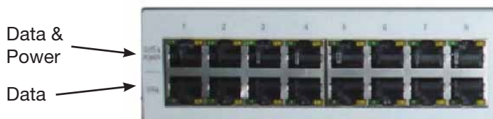
Figure 2: Data & Power (top row), Data (bottom row)
