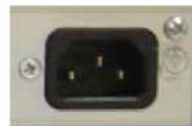
Figure 6: AC Input Connector AC IN: IEC320 inlet 3 pin
